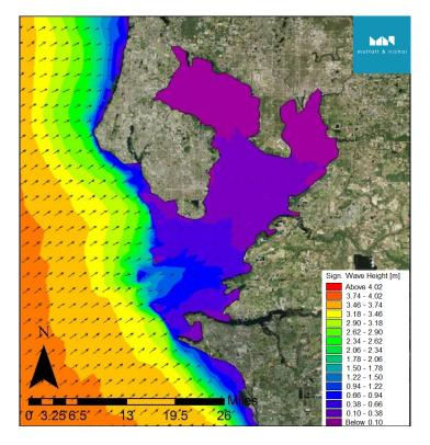
Figure 3 Example of offshore swells propagation throughout Tampa Bay
