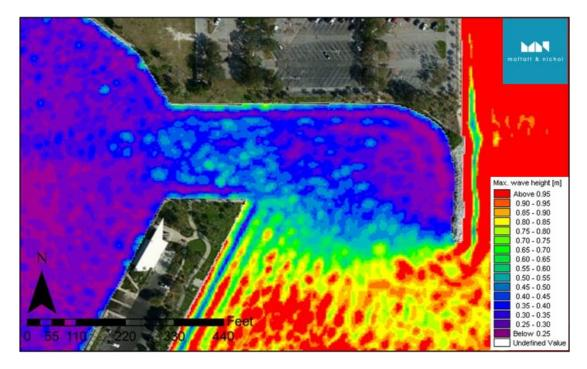
Figure 18 Maximum wave height at the location of the transient docks ( $T_p$ =4sec.  $\theta$ =90°)
