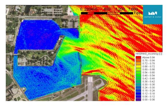
Figure 10 H<sub>s</sub> reduction factor (T<sub>p</sub>=4sec. θ=120°)
