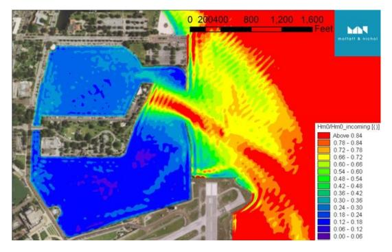
Figure 17 H<sub>s</sub> reduction factor (T<sub>p</sub>=7sec. θ=150°)
