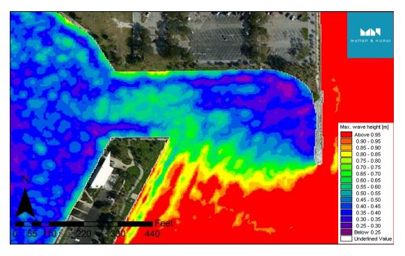
Figure 19 Maximum wave height at the location of the transient docks (T<sub>p</sub>=7sec. θ=90°)
