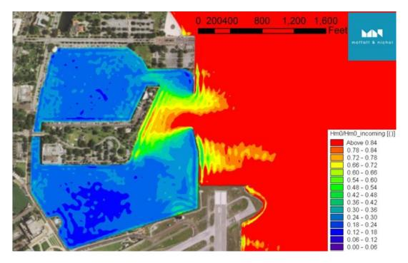
Figure 14 H<sub>s</sub> reduction factor (T<sub>p</sub>=7sec. θ=105°)
