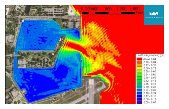
Figure 16 H<sub>s</sub> reduction factor (T<sub>p</sub>=7sec. θ=135°)
