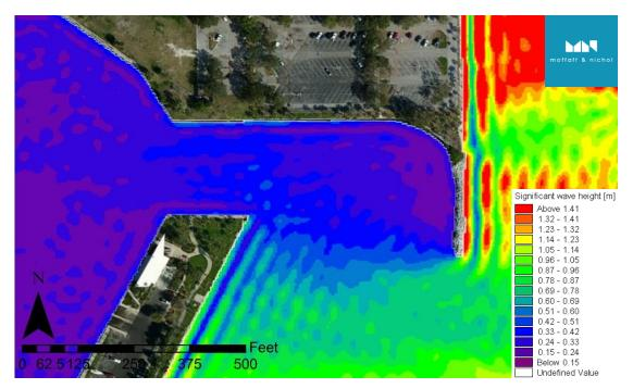
Figure 21 Maximum wave height at the location of the transient docks for the 100-year storm event  $(H_{s \text{ offshore}}=1.5m., T_p=4.2sec. \theta=90^\circ)$
