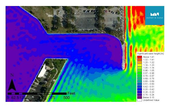
Figure 20 Maximum wave height at the location of the transient docks for the 50-year storm event ( $H_{s \text{ offshore}}$ =1.4m.,  $T_p$ =4.2sec.  $\theta$ =90°)
