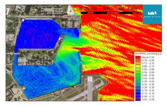
Figure 9 H<sub>s</sub> reduction factor (T<sub>p</sub>=4sec. θ=105°)
