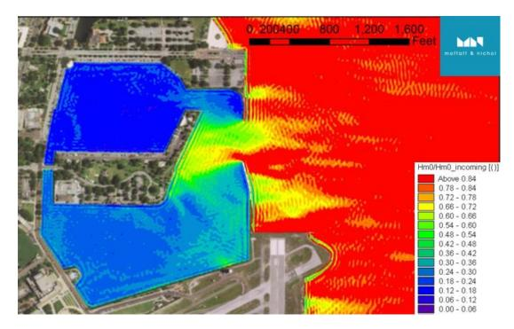
Figure 8 H<sub>s</sub> reduction factor (T<sub>p</sub>=4sec. θ=90°)
