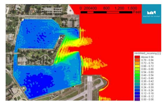
Figure 13 H<sub>s</sub> reduction factor (T<sub>p</sub>=7sec. θ=90°)
