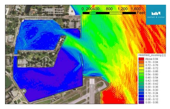
**Figure 12 H**<sub>s</sub> reduction factor (T<sub>P</sub>=4sec. θ=150°)
