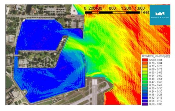
Figure 11 H<sub>s</sub> reduction factor (T<sub>p</sub>=4sec. θ=135°)
